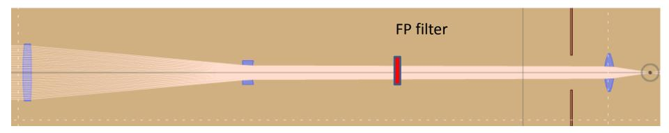
One lens (the refocuser or the ocular) provides converging rays onto the imaging plane
