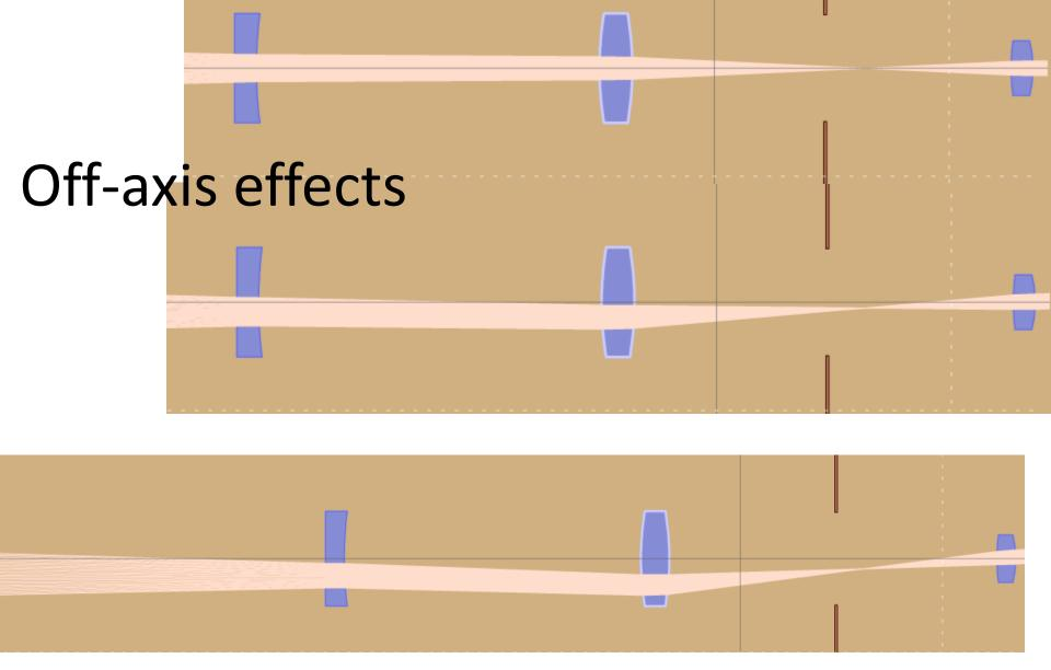
• 0,0.1,0.2 degrees off axis. Near parallel but slanted beam, so will not get same etalon filter response over solar disk
