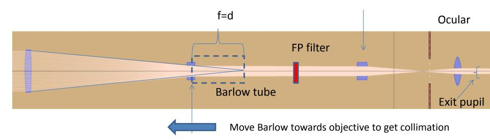
Collimation/parallel rays occurs when Barlow placed within prime focus at a distance **d equal to the focal length f** of the Barlow lens
